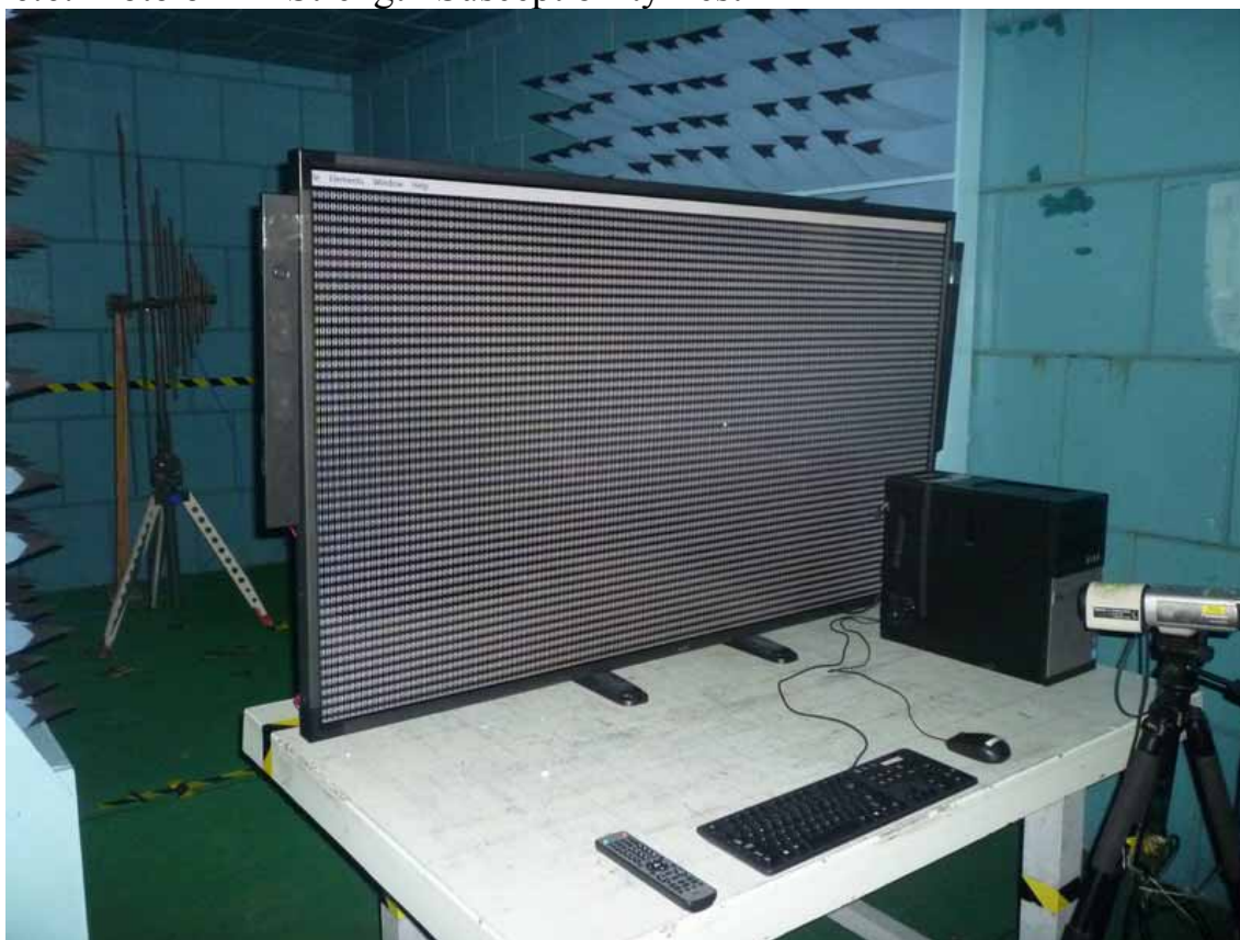
16.6.Photo of RF Strength Susceptibility Test
